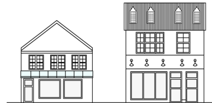
Graphic 1.2 Example depicting first floor storefronts with 70% of the first floor wall area as a glazed display or window.
